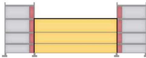
Circulation Diagram 2 Parking and residential floors aligned
